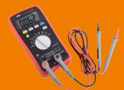
Direct current intensity: 400µA - 10A. Alternating current intensity: 400µA - 10A. Direct current voltage: 400mV - 600V. Alternating current voltage : 400mV - 600V. Resistance : 4000hm - 40M0hm. Continuity with Buzzer Diode test. Frequencies : 5Hz - 50MHz.
