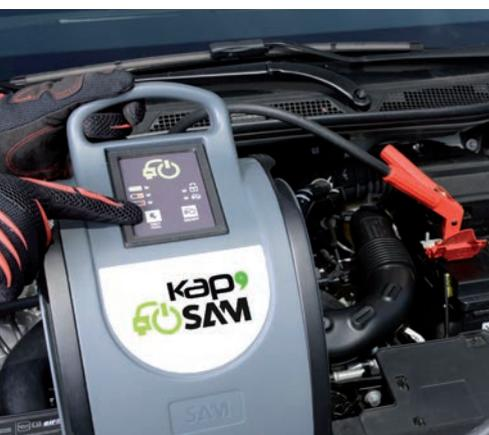
Technically, the Kap'SAM<sup>®</sup> is a device that can produce a large amount of spontaneous power and has an impressive capacitance in the 12V version, with a current of 1600 amps in start mode and a peak current of almost 9000, or a capacitance of almost 500 farads.
